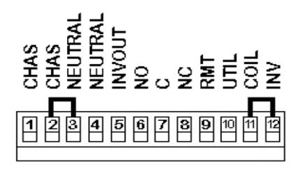
The alarm contact is configured via jumpers on a removable terminal plug on the back of the inverter
